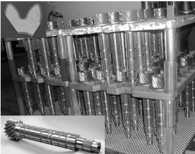
Fig 2 Typical LPC application to transmission axles in a commercial heat treater shop (18MnCr5).
